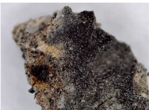
Microscopic image of a weld sample with visible change of colours due to the corrosion of iron added to the mortar – mill scale
